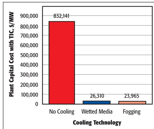
Figure 5. Effect of Cooling Technology on Incremental Plant Capital Cost for the Industrial CT
