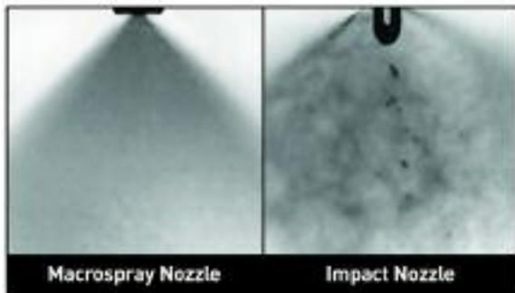
The Macro Spray nozzle (left) provides consistent water dispersion, superior to the impact nozzle's pattern (right), which exhibits voids and rogue droplets.
