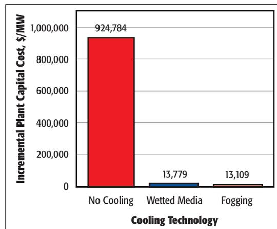
Figure 6. Effect of Cooling Technology on Incremental Plant Capital Cost for the Aeroderivative CT
