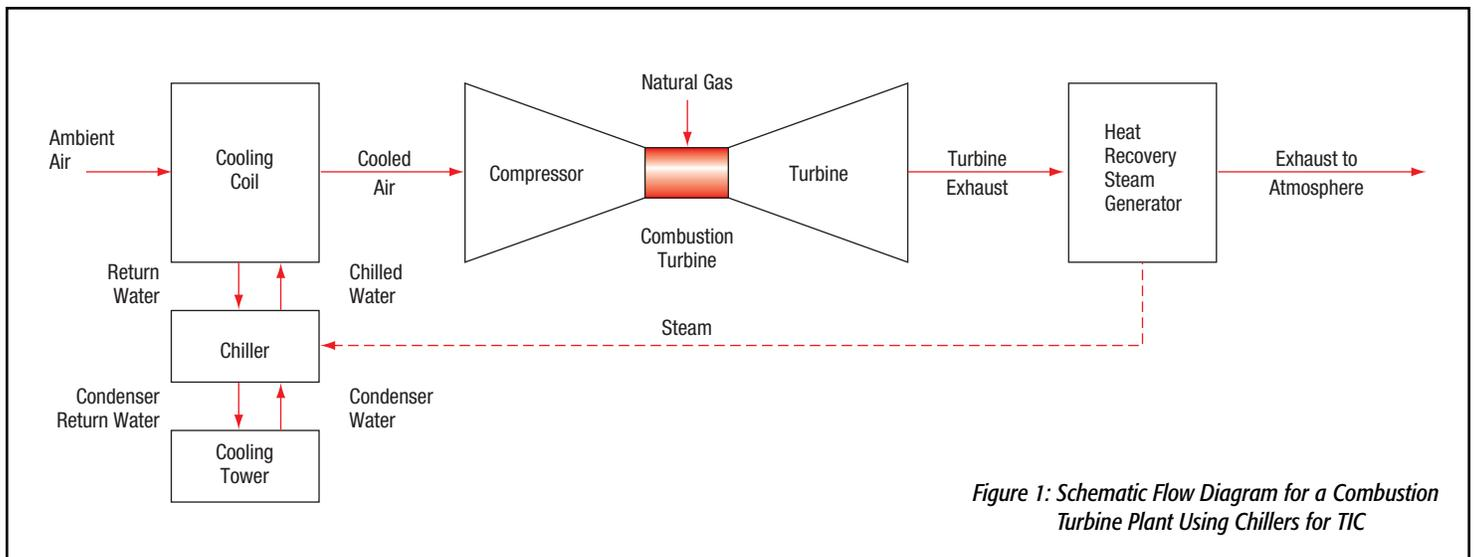
Figure 1: Schematic Flow Diagram for a Combustion Turbine Plant Using Chillers for TIC
