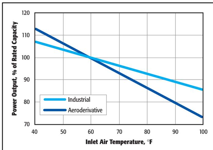
Figure 1: Effect of Inlet Air Temperature on Combustion Turbine Power Output
