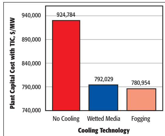
Figure 4 Effect of Cooling Technology on Total Plant Capital Cost for the Aeroderivative CT
