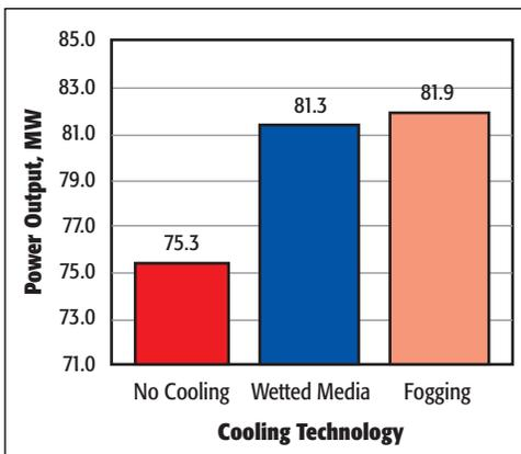
Figure 1. Effect of Cooling Technology on Net Power Output of the Industrial CT
