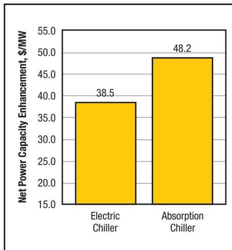
Figure 3: Effect of Chiller Technology on Net Power Output
