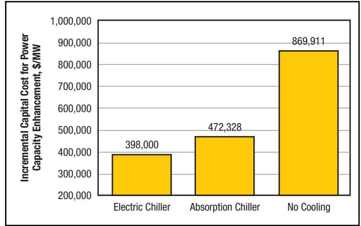
Figure 5. Effect of Chiller Technology on Capital Cost for Incremental Plant Capacity Enhancement
