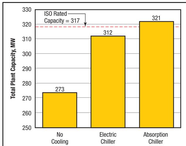
Figure 2: Effect of Chiller Technology on Total Plant Capacity
