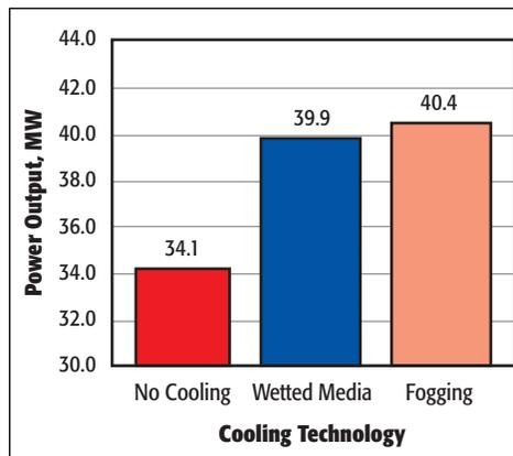
Figure 2. Effect of Cooling Technology on Net Power Output of the Aeroderivative CT
